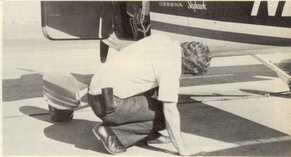
When was the last time you went "on all fours" to check the belly, not only for damage to the structure, but also for excessive oil streaking . . . ?
